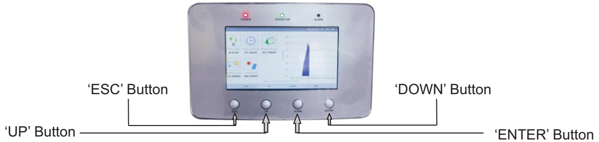
Fig 5 Configuring Inverter Address
